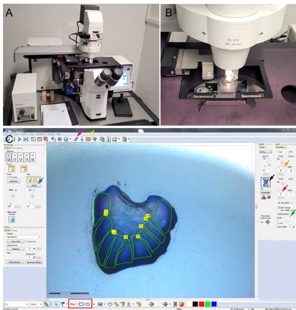
Figure 2. Zeiss PALM microbeam-laser microdissection microscope and PALMRobo 4.8 Pro settings for laser microdissection of Bicyclus anynana larval and pupal wings. (A) Zeiss PALM microbeam-laser microdissection microscope. (B) A closeup of the mounted slide on the microscope. (C) Settings used for laser microdissection of the larval and pupal wing tissues. Magenta arrow: slide holder control; yellow arrow: collection cap control; orange arrow: laser energy; red arrow: laser focus; green arrow: number of laser cutting cycles; blue arrow: intensity for the backlight; and red box: tools for selecting the sections for microdissection.
